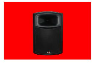
The MK-15 loudspeaker system is a compact device designed to perform in a wide range of public address and sound reinforcement applications. It is a 2Way passive system consisting of one proprietary 15 inch low frequency drivers and a high frequency driver with a 90x60 degrees horn, housed in a vented enclosure.
